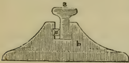
Fig. 227—Represents a cross-section a , of the fish-bellied rail of the Liverpool and Manchester Railway, and the method in which it is secured to its chair. The rail is formed with a slight projection at bottom, which fits into a corresponding notch in the side of the chair b . An iron wedge c is inserted into a notch on the opposite side of the chair, and confines the rail in its place.
